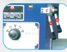
SPEED CHANGE (for KMR-700DS) 1. High or low speed lever (2 stages) Pull for high speed Push for low speed
